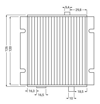
126x105x49 mm (excl. connectors and mounting brackets) 139x130x49 mm (incl. connectors and mounting brackets)
